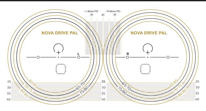
Fitting cross is located 4mm above lens Prism Reference Point
